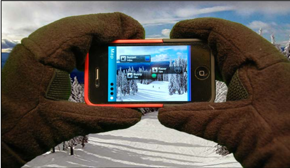
Figure 9: Final Prototype for the iPhone Depicting the gestural navigation, which is operable while wearing bulky gear
